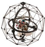
Touch the untouchables with Gimball – a collision-tolerant flying robot that could remain stable after coming in contact with possible deterrent.
